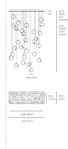
PENDANTS:twenty-eightMOUNTING:white powder coated rectangular canopy 1320mm (52')<br/>x 444mm (17.5') x 53mm (2') deepLAMPING:1.5w LED or 20w xenonCOAX:fixed lengths. 3000mm (10') standard / up to<br/>30500mm (100') maximumMATERIALS:blown glass, braided metal coaxial cable, electrical<br/>components, white powder coated canopyWEIGHT:approximately 66.8kg (147lb)POWER<br/>SUPPLIES:integral
